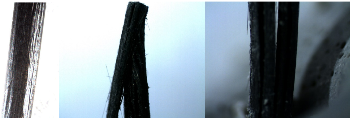
Fig. 4. Composite fibre CF1: before pull-out (on the left) and after complete extraction from concrete matrix M1, with configuration: embedded 20 mm, angle 60 degrees
