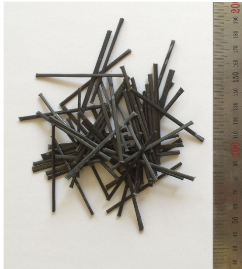
Fig. 1. Composite carbon fibre with 24 000 filaments ( L = 50 mm, d = 1.77 mm)
